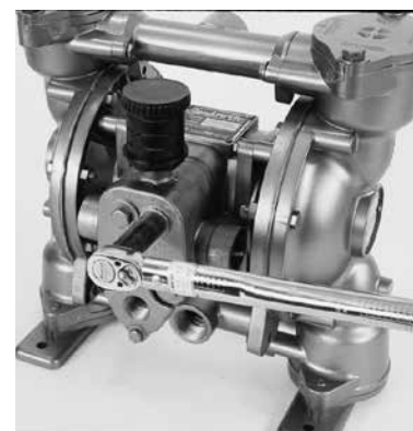
Fig. 8 Torquing the air inlet capscrews
