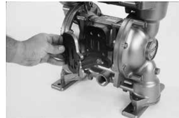
Fig. 9 Pilot valve removal
