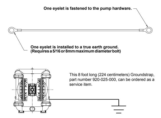
To reduce the risk of static electrical sparking, this pump must be grounded. Check the local electrical code for detailed grounding instruction and the type of equipment required, or in the absence of local codes, an industry or nationally recognized code having jurisdiction over specific installations.
