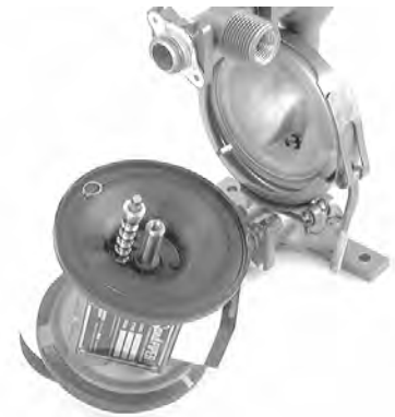
Figure 6: Disassembling the pilot valve.
