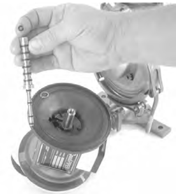
Figure 7: Pilot valve with o-rings.
