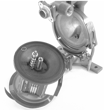
Figure 6: Disassembling the pilot valve.
