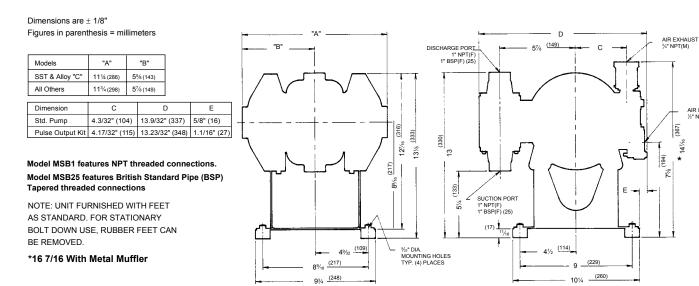
MSB1: 1" NPT(F) SUCTION AND DISCHARGE • 1/2" NPT(F) AIR INLET PORT • 3/4" NPT(F) AIR EXHAUST PORT (NOT SHOWN) MSB25: 1" BSP(F) TAPERED SUCTION AND DISCHARGE • 1/2" NPT(F) AIR INLET PORT • 3/4" NPT(F) AIR EXHAUST PORT (NOT SHOWN)
