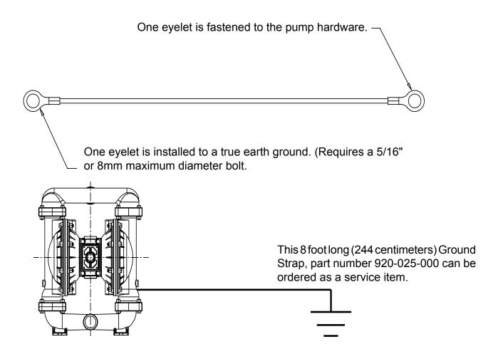
To reduce the risk of static electrical sparking, this pump must be grounded. Check the local electrical code for detailed grounding instruction and the type of equipment required, or in the absence of local codes, an industry or nationally recognized code having jurisdiction over specific installations.
