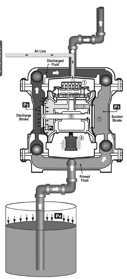
Air-Operated Double Diaphragm (AODD) pumps are powered by compressed air or nitrogen.
