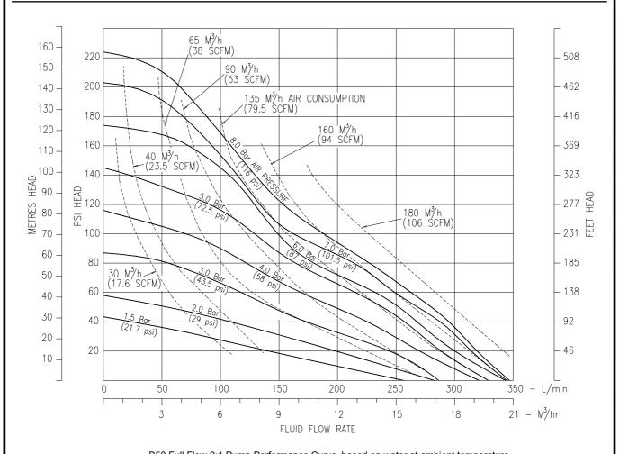
B50 Full Flow 2:1 Pump Performance Curve, based on water at ambient temperature
