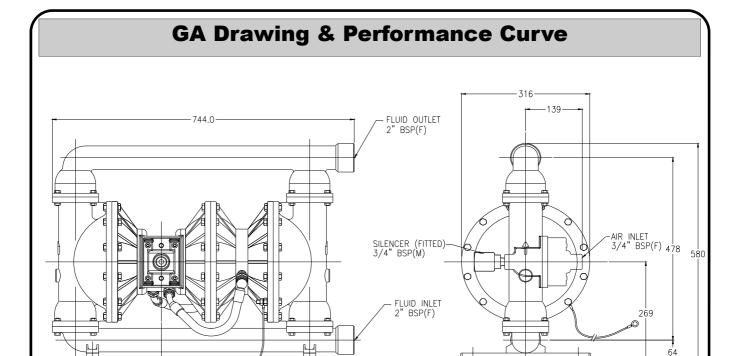
General Assembly B50 / X5005 Full Flow 2:1 Pump :- All dimensions +/- 3mm
