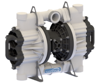
HD20F Non-Metallic Max Flow: 150 GPM (567 LPM) Max Solid Size: 1.8 inch (45.7 mm) ONLY 53 POUNDS (24 kg)
