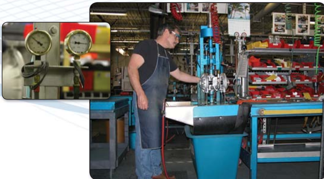
Experienced SANDPIPER assembler monitors pump performance with pressure and vacuum gauges.
